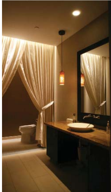
LEFT: two story solar tubes introduce natural light into lower level restrooms. Warm-tone fluorescent sconces illuminate individual stalls and provide flattering facial illumination. Concealed halogen downlights within solar tubes provide sparkle at the lavatories.
